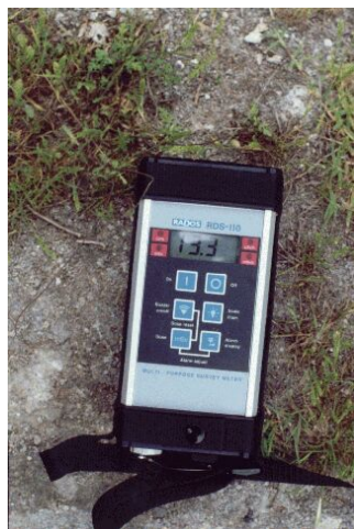
Figure 3. A calibrated survey meter shows the contact dose rate.
