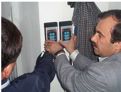
Figure 6. Two survey meters show the dose rates of 142 and 143 micro Gy/h on the wall of the bedroom of one dwelling.
